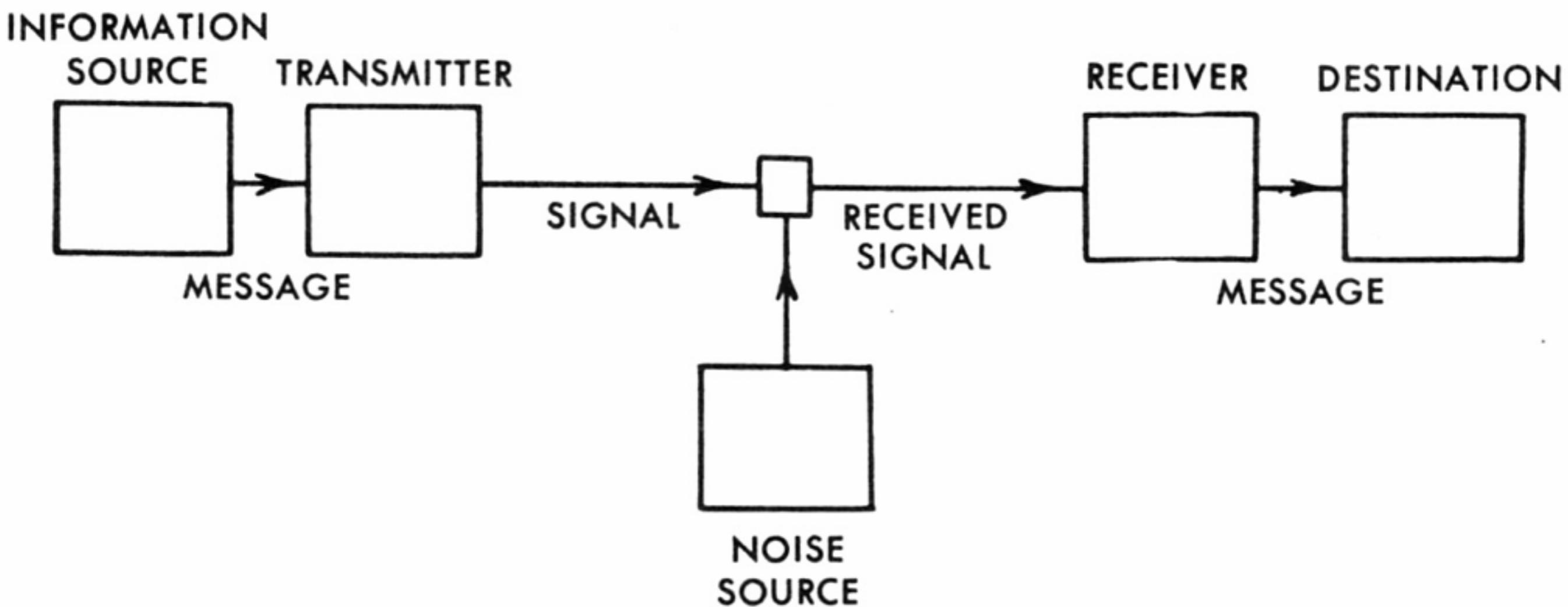
Fig. 1.— Schematic diagram of a general communication system.
