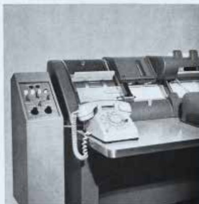
At the data processing center, an IBM Card Punch receives data by phone and automatically punches it into a card, ready for processing.
