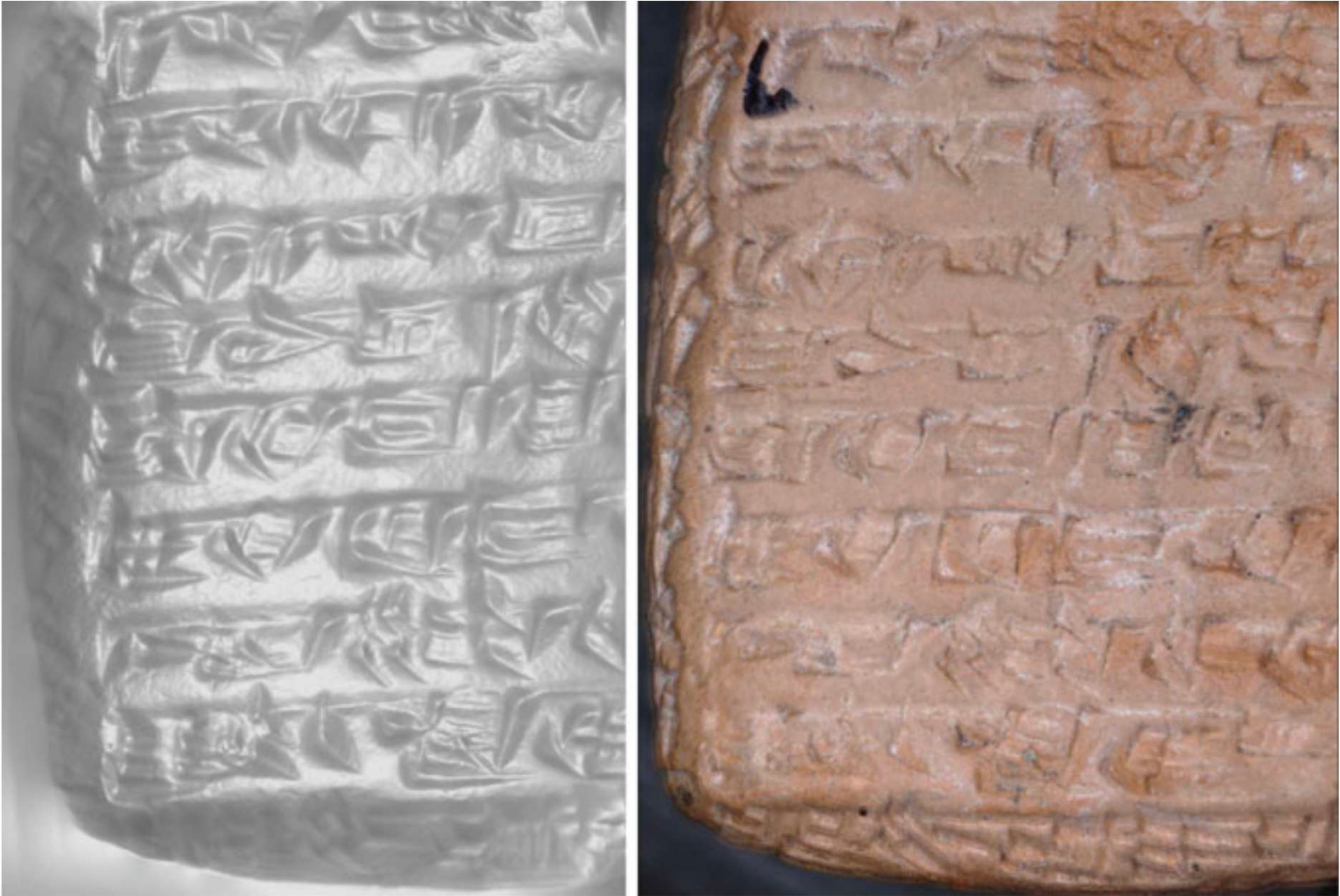
Fig. 2 Digital model of surface topography of cuneiform tablet separated from its colour is rendered in a simulated illumination enhancing shapes of signs (left part of figure). The 3D model is acquired by photometric stereo technique. The same area of the same tablet captured by focus stacking technique of digital photographs is shown for comparison on the right. Such a visualization is capable of substituting a direct contact with the tablet
